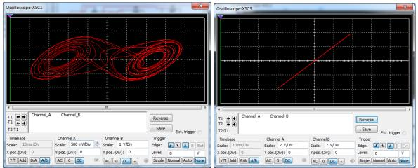
Figure 3. There is no resistance which between the connecting line of master and slave (transmitter - receiver). Form the left is the attractor and from the right the scope in XY mode were in X represent the voltage of C1 and C2 the voltage over C2.
