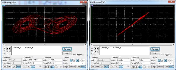
Figure 4. The resistance which connect the master-slave oscillator is  $R=3.5 \text{ k}\Omega$ . As it can been seen there is synchronization.
