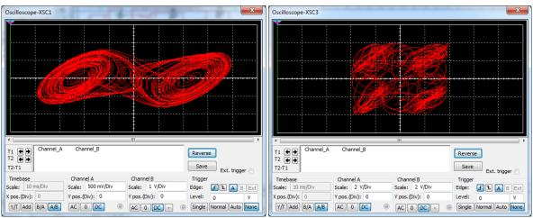
**Figure 5**. The resistance which connect the master-slave oscillator is  $R=10k\Omega$ . As it can been seen there is no synchronization.
