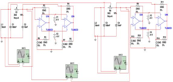
Figure 2. The synchronization of two couple chaotic oschilators.
