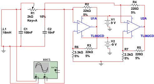
Figure 1: The schematic of the Chua's circuit.
